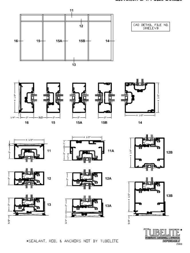
14.08 14000 Series Flush Glaze Isometric Assembly Details
